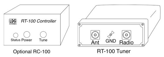
The RT-100 is powered via 12VDC, which is supplied over the same coax cable used for the antenna feedline. A bias tee or optional RC-100 is needed at the radio end of the cable, to inject DC power onto the feedline. Because power is supplied over coax, the existing coax feedline to your antenna is all you need to hook up the RT-100. No additional cables are required in order to run power or control signals to the tuner.
